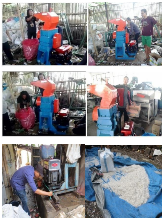
Figure 8. Plastic Shredding Machine Operation Trainin
