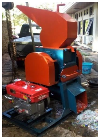
Figure 2. Inorganic waste processing machine
