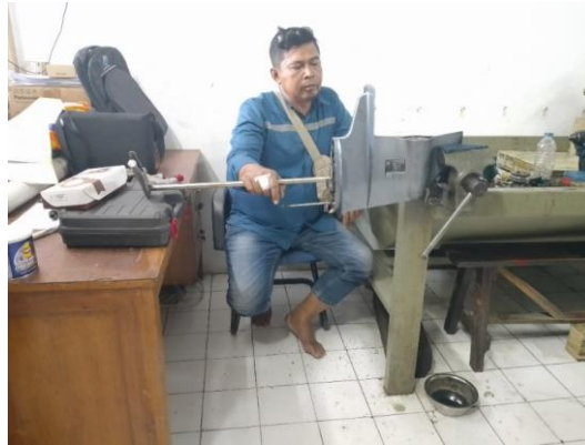
Figure 5. Dismantling the Lower Unit Section
